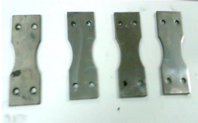
**Figure 2.3** Fatigue Testing Specimens
