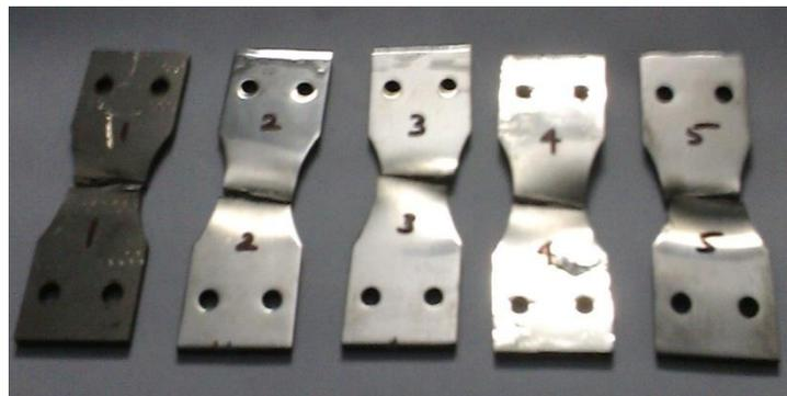
Figure 3.6 Specimens after bending fatigue testing
